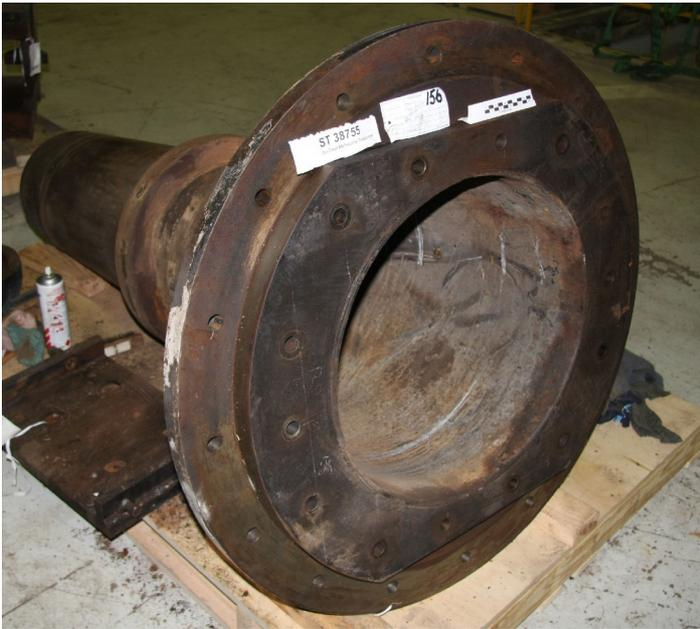
Staff from the Scienceworks engineering workshop also discussed trying to push the flange off with large hydraulic jacks. Our greatest concern, which led to this idea also being abandoned, was the fear of cracking the original axle casting, structurally weakening it and rendering it unreparable.
