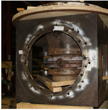
North face, showing the spigot that locates the friction-relief apparatus
