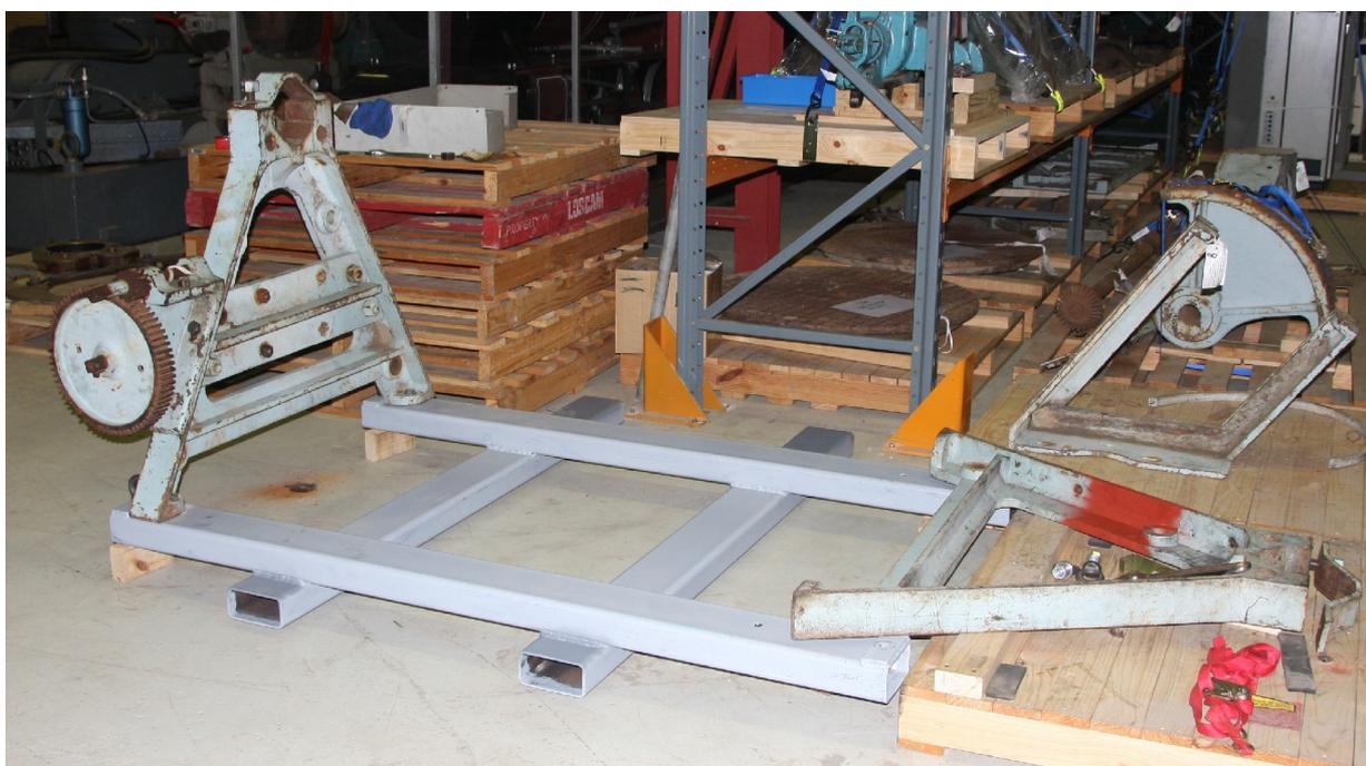
Now all we have to do is reassemble the MGPM (including the manufacture of a few missing parts, and replacement of the bearings) and put it on top of that - and as you can see, by the time I brought the camera in, the trial fittings for assembly on the stillage had already begun. The finished machine will be mechanically in working order but, despite its name, it will not actually be used for grinding and polishing any mirrors.
