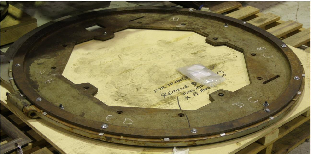
The Declination Axis Clamp Disk, long ago broken into 5 pieces but here re-assembled, pulled tight by the Clamp Ring itself and bolted to a plywood board. For safety and conservation reasons, a new casting is being made and will be machined to faithfully match the original in all details, except that the central hole will be circular instead of octagonal
